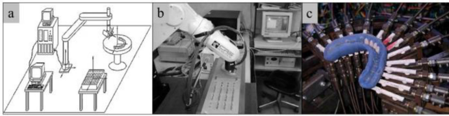
Fig. 8. Tooth arrangement robots (a) serial robot with normal grasper [89], (b) serial robot with tooth-caps [84], (c) multi-manipulators [90].
